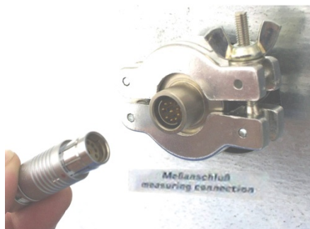
Figure 22: Measuring connection (12) with measuring access port
